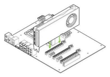
Note: Install the SupremeRAID<sup>™</sup> card into the primary x16 PCI Express slot. The SupremeRAID<sup>™</sup> SR-1010 is dual-slot card and covers the adjacent slot. The SupremeRAID<sup>™</sup> SR-1000 and SupremeRAID<sup>™</sup> SR-1001 are single-slot cards. For more information, see <u>NVIDIA RTX Ampere Architecture-Based Graphics Card</u> <u>User Guide</u>.
